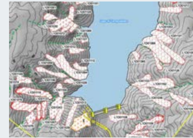
Campolattaro Dam | Asea Benevento, Italy Hydrogeological and Landslide Assessment
